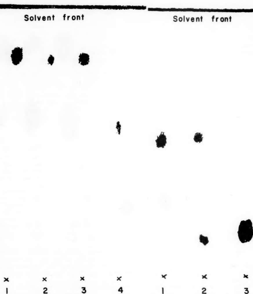
FIG. 3 ( left ). Paper chromatogram of tryptophan derivatives, developed with a solvent consisting of the alcoholic phase from a mixture of n -butyl alcohol, acetic acid and water (80 : 20 : 10, v/v), and sprayed with Ehrlich's reagent. 1. Synthetic succinyltryptophan. 2. Synthetic malonyltryptophan. 3. Extract of tryptophan treated spinach leaves. 4. Synthetic oxalytryptophan.
